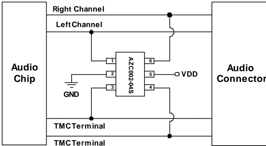
Fig. 4 ESD Protection scheme for audio interface by using AZC002-04S.
